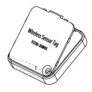
Step 3. Close the lid by pushing down where the hooks (2~4) are, one at a time
