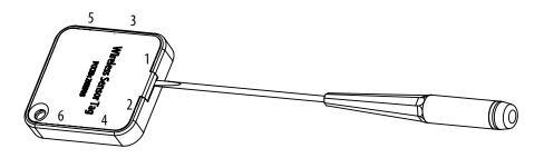
**Step 2.** The circuit board is fitted (without any glue) front-side down in the casing. Use the screwdriver/chisel to remove the board.
