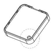
Step 2. Insert the two hooks (1) at the bottom edge of the lid into matching grooves in the case
